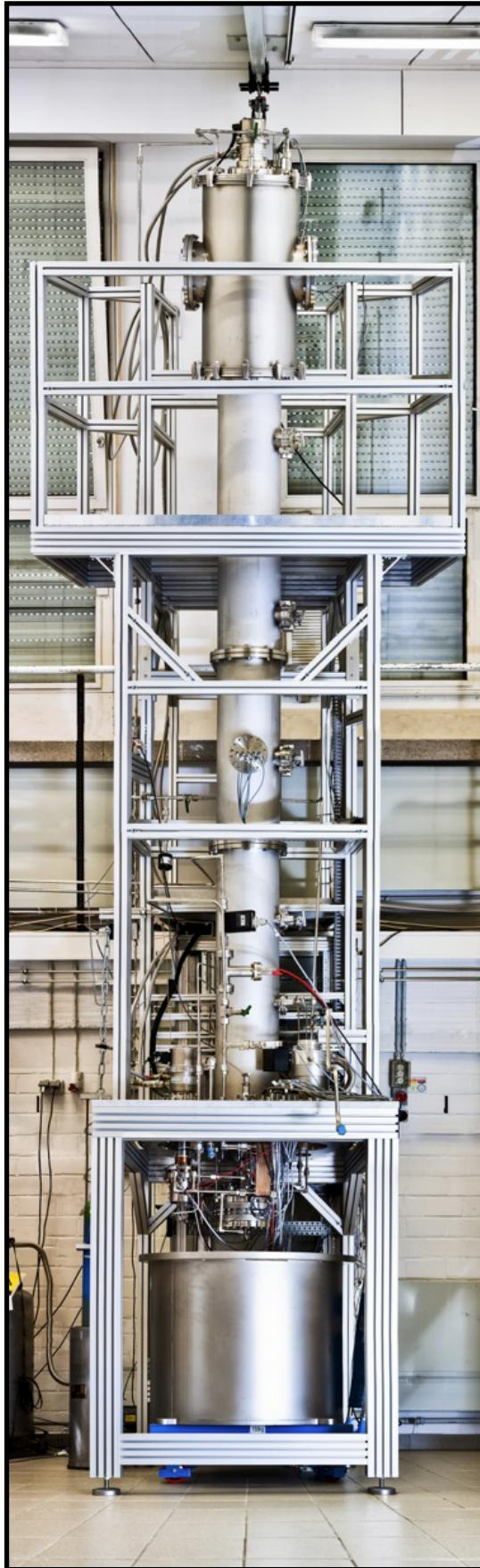
*DarkSide Cryogenic distillation column for purification of  $^{39}\text{Ar}$*
